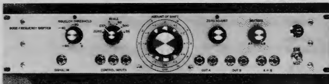
Fig. 3. The front panel layout of the Model 735 Bode frequency shifter.
