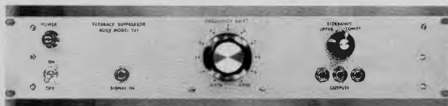
Figure 9. A front panel layout of anti-feedback frequency shifter.
