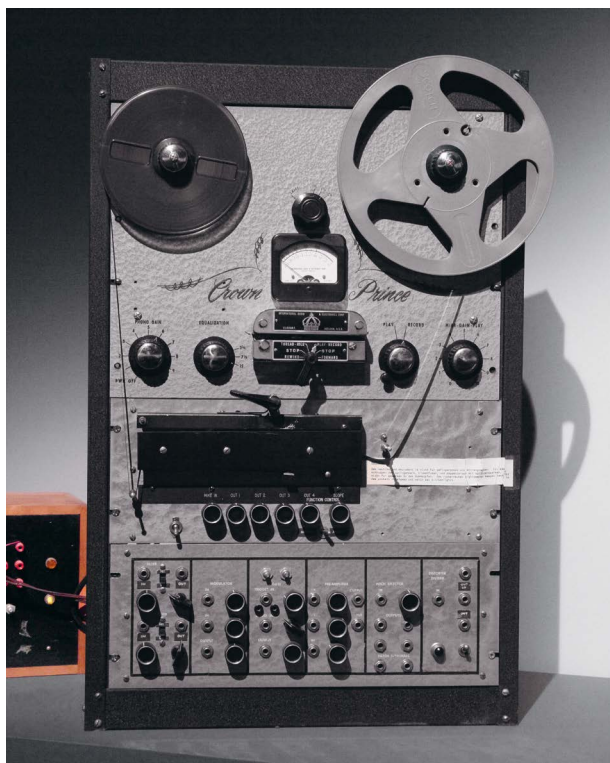
Harald Bode, Audio System Synthesizer with tape deck at top, tape-loop reverberation below, and plug-in modules at bottom, 1960, exhib. view, Harald Bode: Tone Color – Known and Unknown Sounds , Burchfield Penney Art Center, Buffalo State College, Buffalo, NY, 2011.
